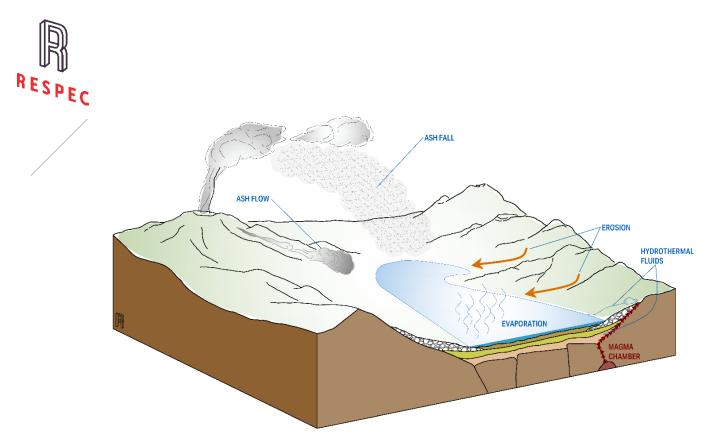
Figure 8-1. Illustration Showing Modes of Lithium Emplacement Believed to Have Occurred at the Property.
