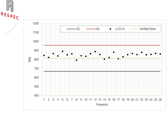
Figure 11-1. CRM Standard MEG.Li. 10.14 Geochemical Laboratory Results.
